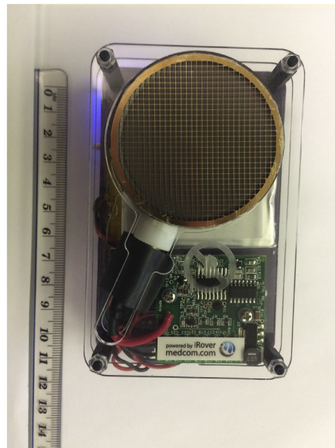
Fig. 2. These images show the front and back of the bGeigie Nano, and is the current handheld unit for contributing radiation observations to the Safecast database. This is the fifth generation of the bGeigie handheld sensor, which was released in 2013. (bGeigie Nano images courtesy of PSU's Geoinformatics and Earth Observation Laboratory).
