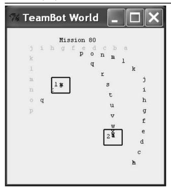
**Fig. 6** Track of the human (starting at top) and the robot (starting at the bottom) avoiding a conflict by simulating the human's decision-making. Both began at their respective "a" locations and patrolled counter-clockwise until the alarm occurred at "p". The robot then, in accordance with the shared plan, determined where the human would go by simulating the human's decision-making using its own knowledge and therefore immediately started toward the other station
