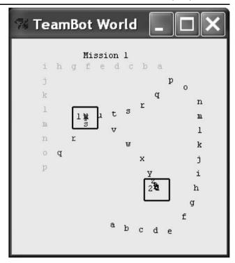
**Fig. 5** Track of the human (*starting at top*) and the robot (*starting at the bottom*) "manning" two guard stations (*numbered squares*) with a conflict. Both began at their respective "a" locations and patrolled counter-clockwise until the alarm occurred at "p." Then both moved toward guard station #1 until, at step "u," the robot detects the conflict and goes to station #2
